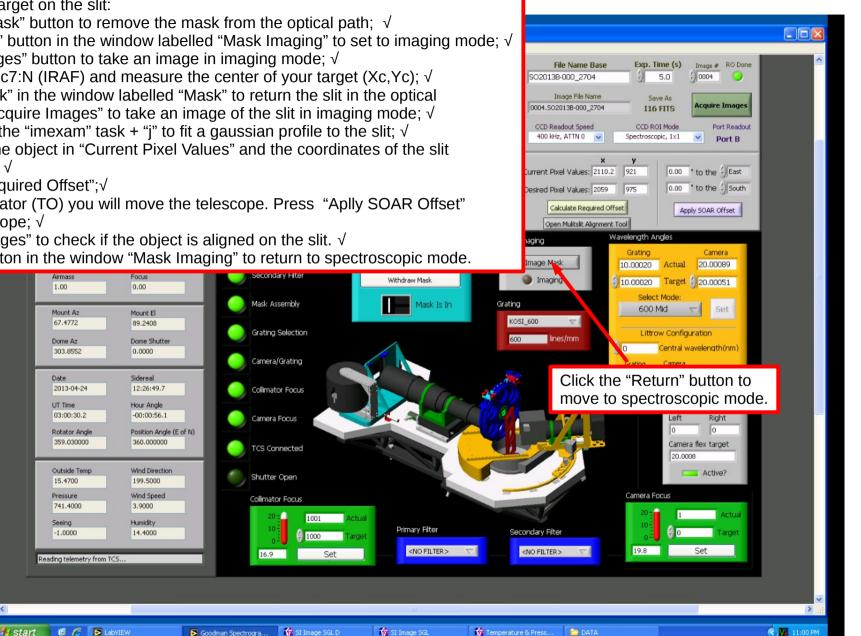
Procedure to center the target on the slit:
